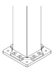
i. Connect post to base using 3/8"-16 x 1" flat head socket screws (x8). The post plate aligns with the recessed cutout in the base. Repeat for other post(s).
