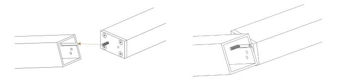
iv. Set desired track angle (flat orientation shown below). This orientation can be changed at any time (see 'Post Assembly'). Insert 3/8"-16 x 1-1/2" hex bolt with 3/8" washer into the plate hole when the appropriate hole in the post is aligned. Repeat on other side of the track supporting beam.
