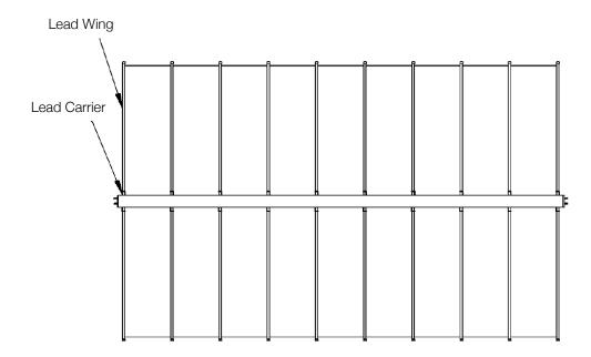
i. Raise wing into carrier assembly. Align holes in wing with holes in carrier assembly.
