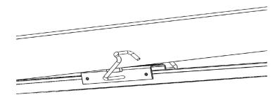
iii. Rotate G-clips downward until they lock into position.
