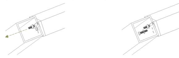
Hold the track supporting beam and slowly release the nut on the protruding thread until rotation is possible
