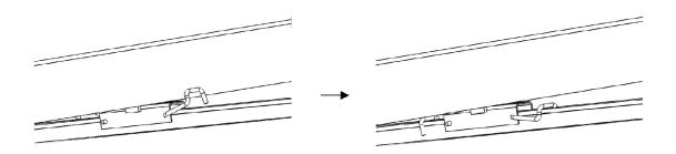
Notice the direction of the G-clips on each side of the drive beam are different.
