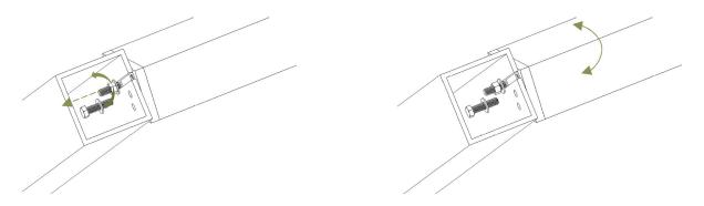
Rotation can be done with the canopy still attached but it is recommended that it be retracted in the <u>middle</u> of the track supporting beam.
