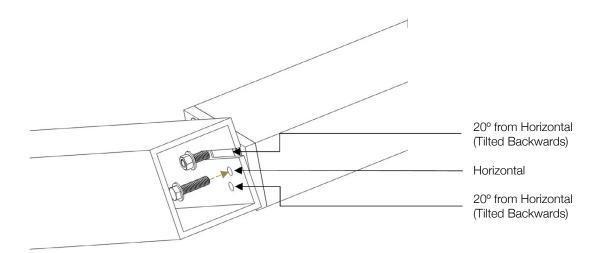
v. Ensure both the bolt inserted in Step 2-iv as well as the nut fastened onto the protruding thread in Step 2-ii are tightened fully and is done on both ends of the track supporting beam.
