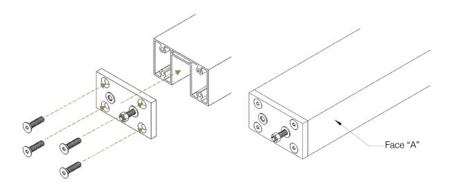
Ensure protruding threads on both rotation plates are adjacent to the same face. Ex: Protruding threads adjacent to Face "A"
