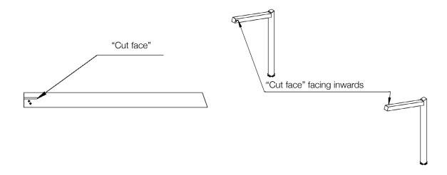
Secure arms in place by installing washers (x4 per arm) and 3/8"-16 hex nuts (x4 per arm) from inside the posts.
