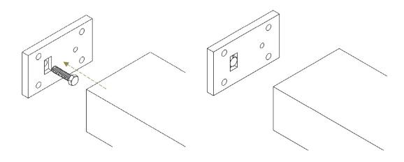
Then, secure the rotation plate onto the track supporting beam using  $3/8"-16 \times 1-1/2"$  flat socket cap screws (x4). Add a 3/8" washer and loosely thread a 3/16" nut until the nut is just on the protruding thread. Repeat on the other side of the track supporting beam.
