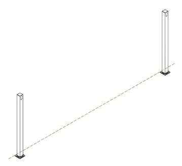
iii. Once the bases are aligned the distance between the inside of the posts should equal the total track supporting beam length (track supporting beam + rotation plate) +1/4".
