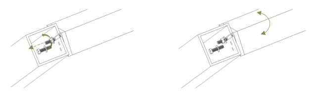
Tighten nut and bolt to secure in place (Canopy Tilted Forward position shown above)
