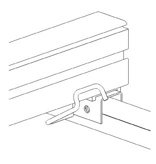
4. Secured wing to carrier assembly
