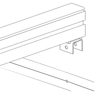
3. Rotate the G-Clip downward to lock into position
