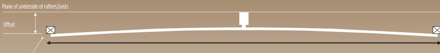
The ideal stabilizer is a 2x2 or 2x4. There should be some stress on the wing from the stabilizer to ensure all movement in the wind is contained. Locate the stabilizers where they just touch the top of the wing, then bring them down approximately 1/4" to preload them.
