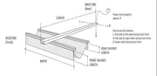
Note: All dimensions are actual desired tip to tip of the beam or wings
