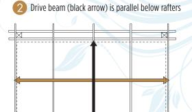
**LENGTH** of drive beam is inside face of beam to inside face of opposite beam LESS 1/4" for clearance
